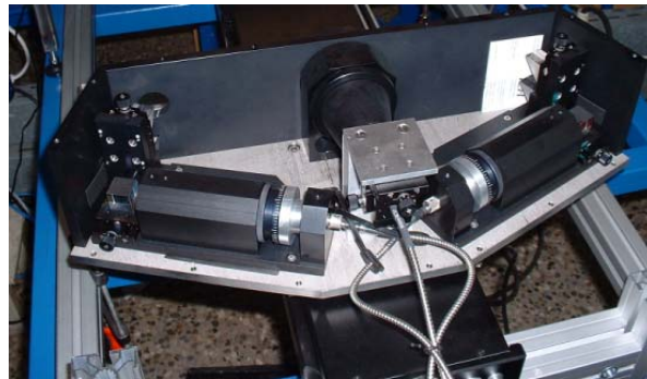
Figure 3: Special LDA realisation for PTB Berlin (measurement volume length 100 \mu m, measurement error < 0,1%)
