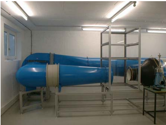
Wind tunnel D320 with LDA for profile measurements
